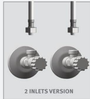
**MAKE SURE THAT THE FILTERS ARE INSTALLED BETWEEN THE FLEXIBLE PIPE AND THE SHUT OFF VALVE/ANGLE VALVE (NOT SUPPLIED).**
